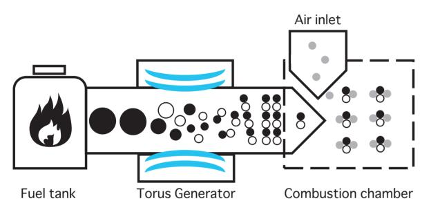
Methane molecules can absorb electromagnetic radiation of a certain wavelength. When subjected to continuous energy, the molecules vibrate more intensely to absorb the energy. This intense vibration creates more friction with oxygen molecules, thereby accelerating the combustion reaction and increasing the flame temperature to improve combustion efficiency.
